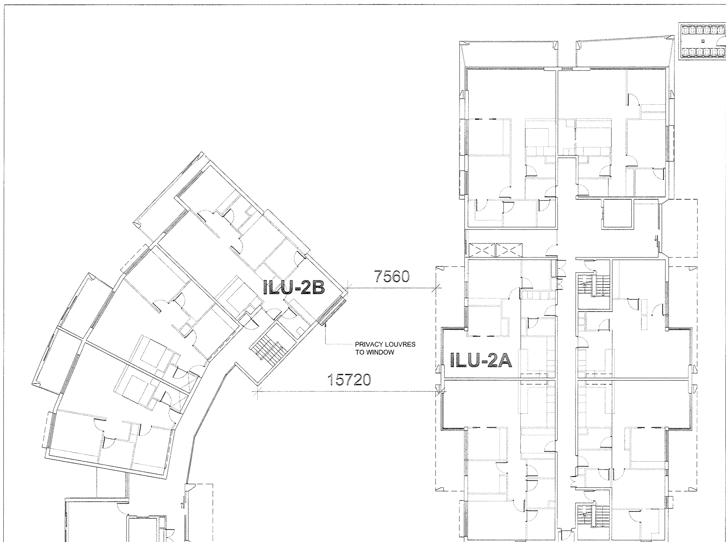
02 BUILDING SEPARATION - ILU 2A & 2B 1:200 @ A1, 1:400 @ A3
